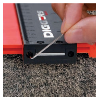
3. The tension of the locking system can be adjusted.
