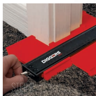
2. Secure the shape with the locking system.
